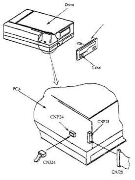
Figure 1-30. Cable Connection
